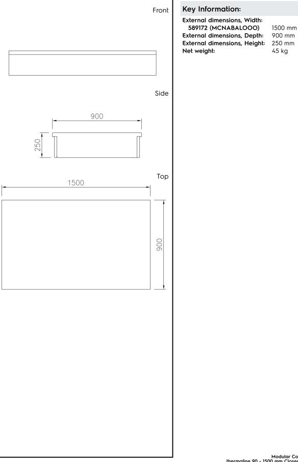
Modular Cooking Range Line thermaline 90 - 1500 mm Closed Work top, 1 Side
